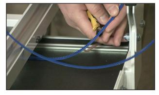
6. At both ends of the blue Flexirack, use two of the small metal clamps (see Parts List, item B) to hold the ends firmly in place. The clamps have a hole through the center and a lip on one end. The lip should be on the side opposite the blue Flexirack. Place the clamps where they will be attached and drill pilot holes using the 3/32-inch drill bit and then use a Phillips screwdriver to fasten the clamps on both sides of the Flexirack to the table.
