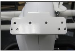
3. Use the four M4x7mm hex screws (provided). Insert them into the Pro-Stitcher bracket and the Infinity front display bracket. Loosely tighten all four screws with a 3mm Allen wrench and then fully tighten them.
