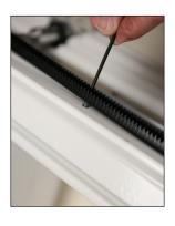
11. Tighten the fourth screw in the slot at the back end of the black rack.
