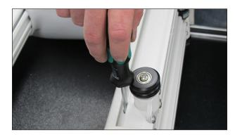
7. Insert three M4 x 12 socket-cap low-profile screws -- one into each of the three holes indicated in the photo. Partially tighten them, leaving them about 1/4 inch out.
