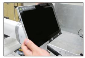
5. Locate the USB cable provided with Pro-Stitcher (see Parts List, item J). Connect one end to the USB port on the tablet computer and the other end to the USB port on the side of the Infinity.
