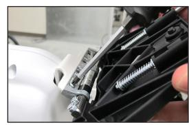
4. Place the tablet computer into the Pro-Stitcher computer bracket. The top part of the bracket is spring-loaded so you can widen the opening enough to get the tablet computer in place.
