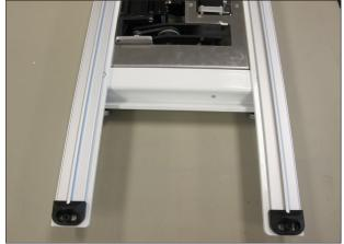
2. Place the Pro-Stitcher carriage on the frame. Starting at one end of the table, begin mounting the blue Flexirack to the front of the table while aligning it to the front white gear on the carriage.
