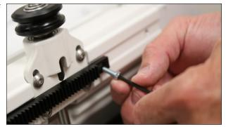
12. Turn the Infinity upright and place it on on the Pro-Stitcher EZ Carriage. Ensure that the white Y-rack gear engages with the black Y-rack. You may need to manually engage the EZ carriage using the manual engagement tool provided.
