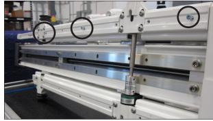
8. Attach the Y-rack black rack (see Parts List, item F-2): Slide the notched end into the end cap and line up the three keyholes in the black rack with the three low-profile screws from step 7.
